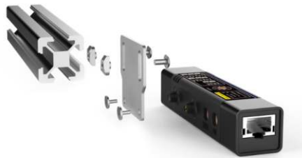
Figure 17 Schematic diagram of sensor installation orientation
