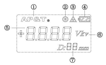
①Corporate trademark ②Holding key open mark ③Test distance positioning mark ④Power display mark
