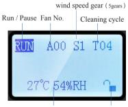
Temperature and humidity Unlock / Lock ( The temperature and humidity sensor is located inside the product )
