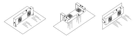
While using the ionizing air blower, the mounting bracket should be fixed on a solid and flat surface (such as a wall or a shelf) with screws or bolts. The angle of the ionizing air blower can be adjusted by the knobs on the two sides of the bracket to achieve the best antistatic effect.
