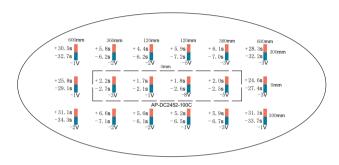
Test standard: ANSI/ESD.STM3.1, SJ/T 11446—2013 Test instrument: Trek 157 static tester Test voltage: ±1000V → ±100V attenuation Test environment: humidity 50±5%; temperature 23±3℃
