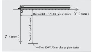
Test standard: ANSI/ESD.STM3.1, SJ/T 11446—2013 Test instrument: Trek charge plate tester Test voltage: ±1000V → ±100V attenuation Test environment: humidity 50±5%; temperature 23±3℃
